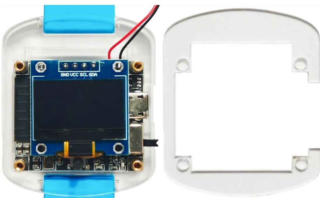
7、Install the corresponding picture shell.
