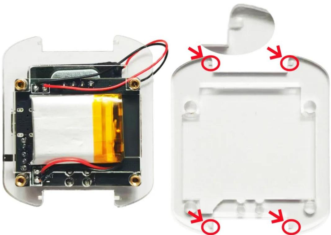
3、Mount the corresponding picture shell onto the back of the circuit board and secure it with M2 screws. (Note the direction of the shell)
