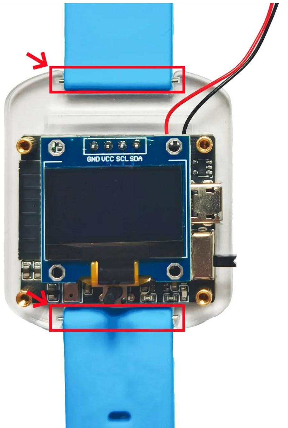
5、Install the corresponding picture shell.
